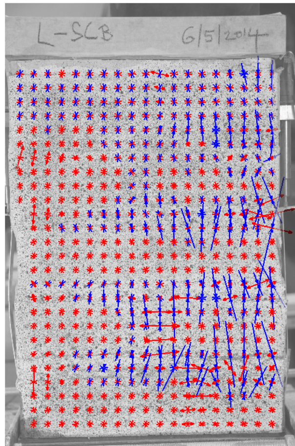
Figure 2.22: Direction and magnitude of principal strains; L-SCB pier in 410 seconds of the test.
