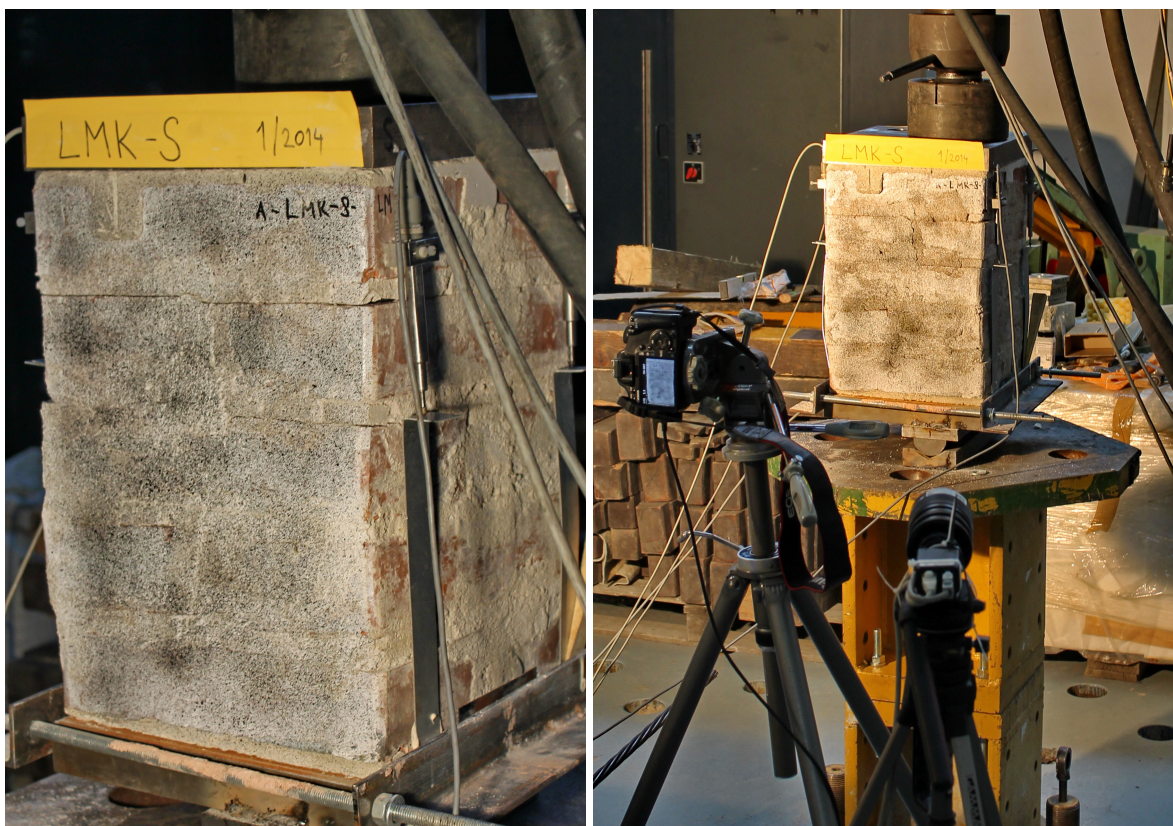
(a) Contrast pattern and attached extensometers
